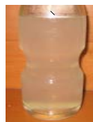
Vac. Btms. after Rinsing Emulsion
